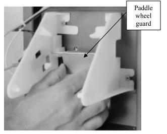
Pull the stainless steel paddle wheel guard from the slot that is cut into the chute...
